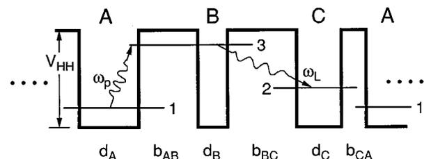
FIG. 1. One period of heavy-hole valence band diagram of superlattice. Hole energy increases in the upward direction.  $V_{\text{HH}}$  is the heavy-hole valence band offset. Indicated are well and barrier widths, subband levels, and pump ( $p$ ) and lasing ( $L$ ) transitions.
