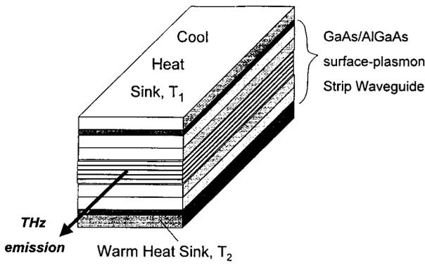
FIG. 2. Perspective view of the Fig. 1 laser.
