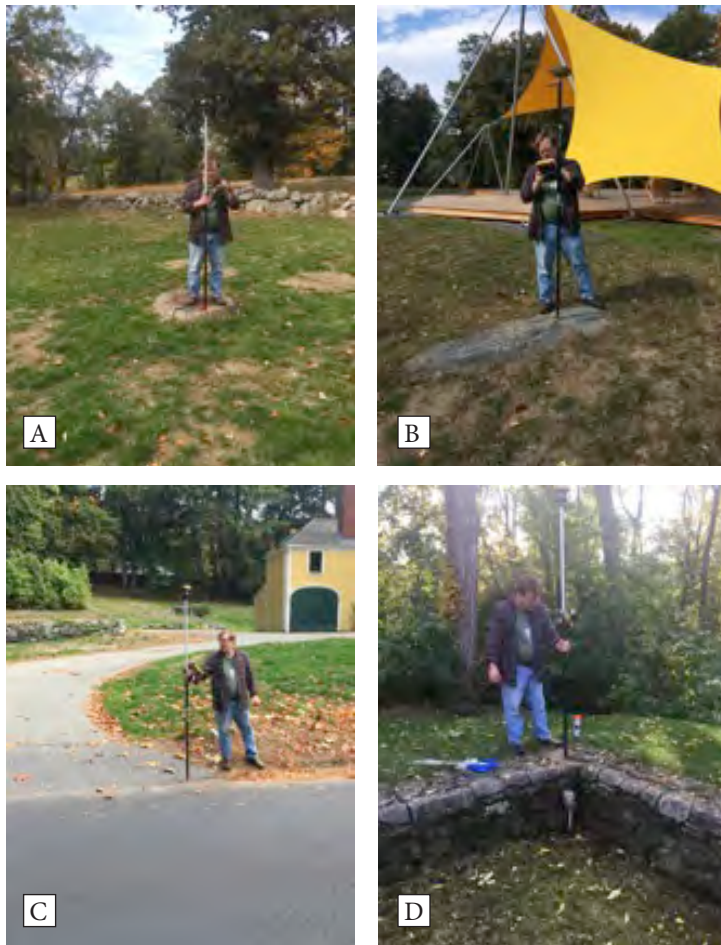
Figure 5. Photographs of some of the land-survey benchmarks listed in Table 1. A) Manhole; B) Hillrock; C) Driveway; and D) Foundation Point.
