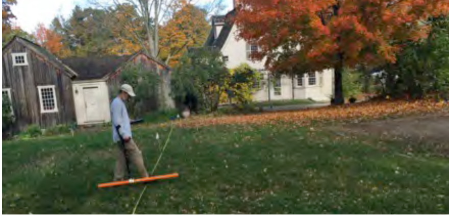
Figure 12. Photo of FDEM surveying with the CMD Mini-Explorer. The tented area is bare ground at the far right.
