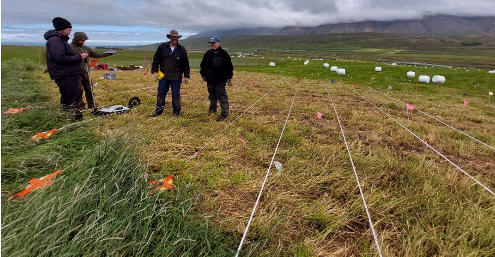
Figure 13. Photograph looking north of the Mala X3 equipped with a 450 MHz antenna at 20 cm transect spacing. The utility line is marked with pink flags.
