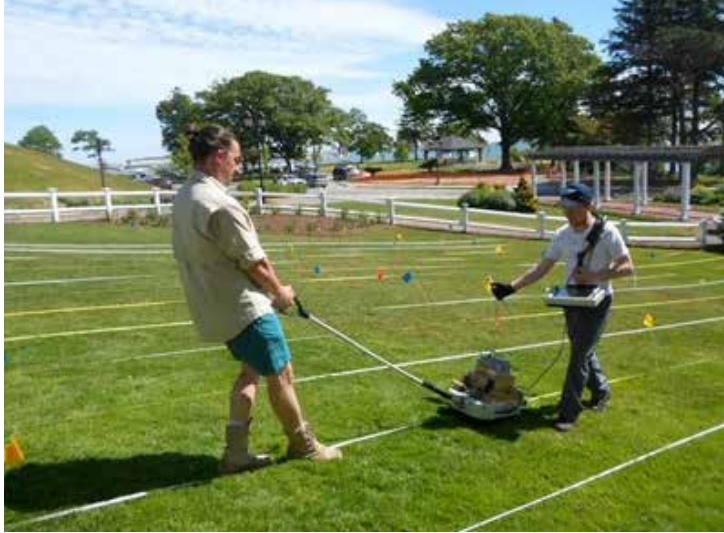
Figure 16. Survey in process: left) GPR surveying with the Mala X3 equipped with a 500 MHz antenna; right) FDEM surveying with the CMD Mini-Explorer.
