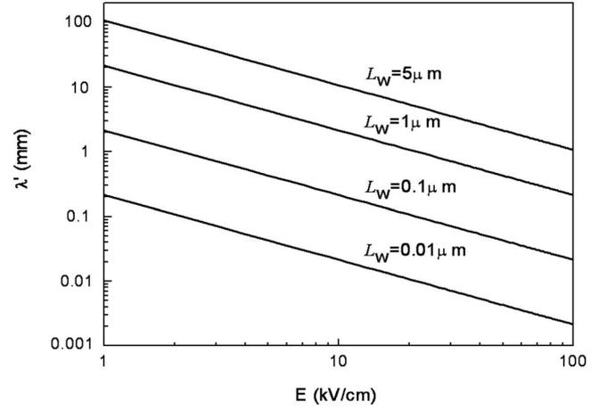
FIG. 2. Emission spectra for different wrinkle periodicities.
