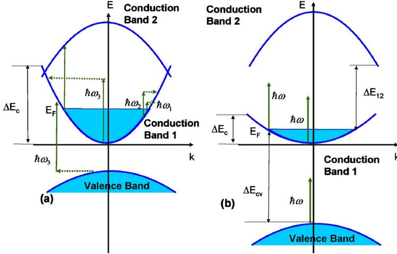
FIG. 1. (Color online) Absorption of electromagnetic waves in metal. (a) The low frequency  $\hbar\omega_1, \hbar\omega_2$  radiation is absorbed by free carriers inside the lowest conduction band, while the higher frequency  $\hbar\omega_3$  radiation is also absorbed by interconduction band transitions. (b) If the photon energy falls into the gap between two conduction bands the absorption cannot take place, while the dielectric constant can still be negative.
