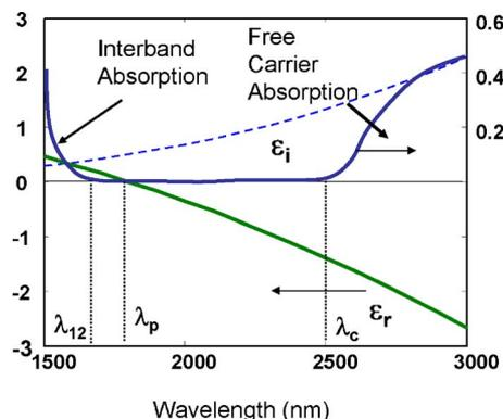
FIG. 3. (Color online) Real and imaginary parts of the dielectric constant for bcc Na with lattice constant of 8Å. The dashed curve shows  $\varepsilon_i$  in Drude approximation with a scattering constant of  $\gamma = 10^{14} \text{ s}^{-1}$ .
