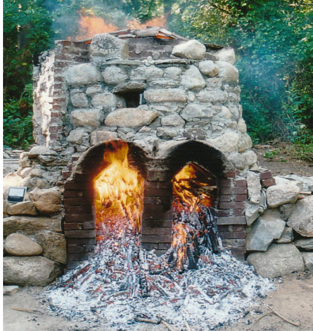
Figure 10. Simple Updraft Kiln in Reduction (Courtesy of Kristen Peltonen and Plimoth Plantation).
