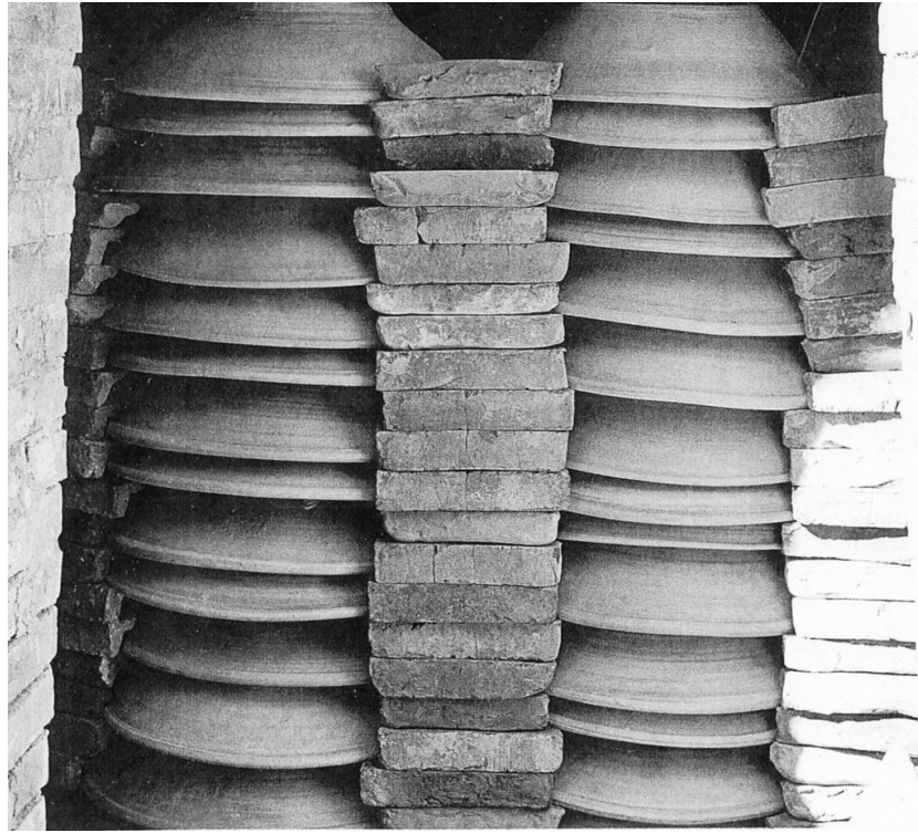
Figure 21. Reproduction kiln at Old Sturbridge Village stacking milkpans with triangular shelves (Worrell 1982:Figure 29).
