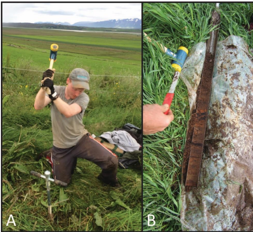
Figure 8. Hammer-percussion Eijkelkamp bi-partite gauge auger A. Core hammering. B. Core cleaning.
