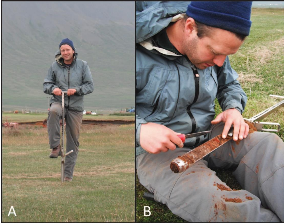
Figure 7. JMC Backsaver Core. A. Core insertion B. Core cleaning.
