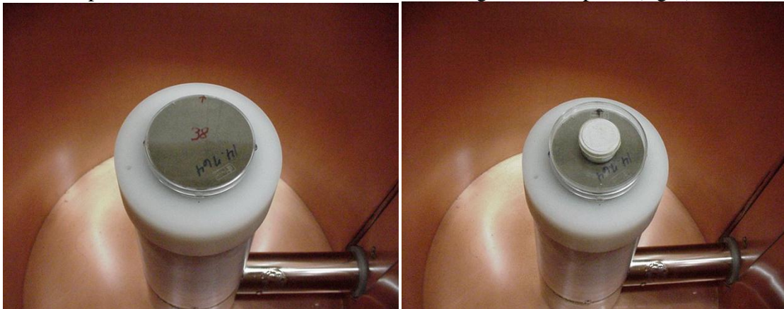
Figure III.1. Photographs of a sample measured on the LEGe detector (left) and the same sample with the button standard for determining self-adsorption (right).
