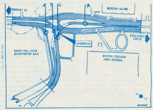
CAMPUS UNDERPASS — Construction will begin next spring on tunnel under Morrissey Boulevard to serve traffic from Kosciuszko Circle to UMass-Boston, due to open next September. Underpass will be 400 feet long, 32 feet wide and have four-foot thick cement base because of high water table. Traffic southbound will cross boulevard at new traffic lights. State Dept. of Public Works took over project from MDC and hopes for 70 percent Federal reimbursement.
