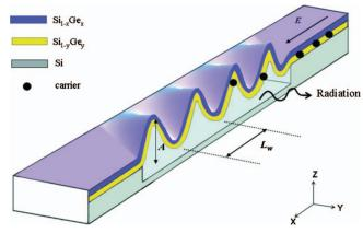
FIG. 1. (Color) Schematic plot of the wrinkled pattern. Holes (solid circle) travel through a sinusoidal trajectory when a voltage is applied across the wrinkled pattern.
