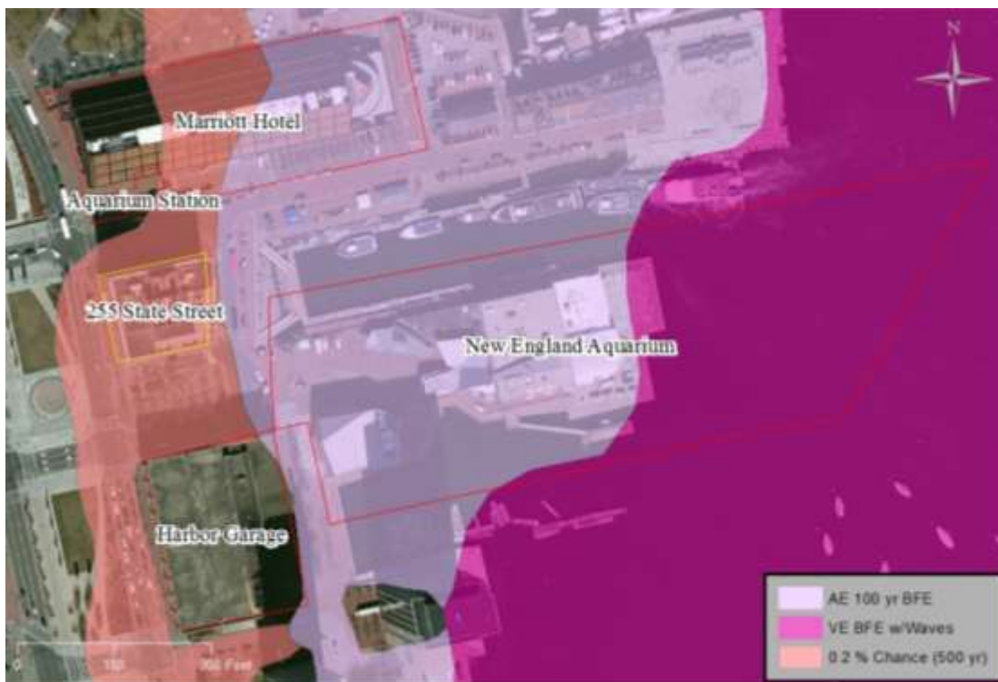
Figure 12. Estimated current 100-year flood zone (Federal Emergency Management Agency)
