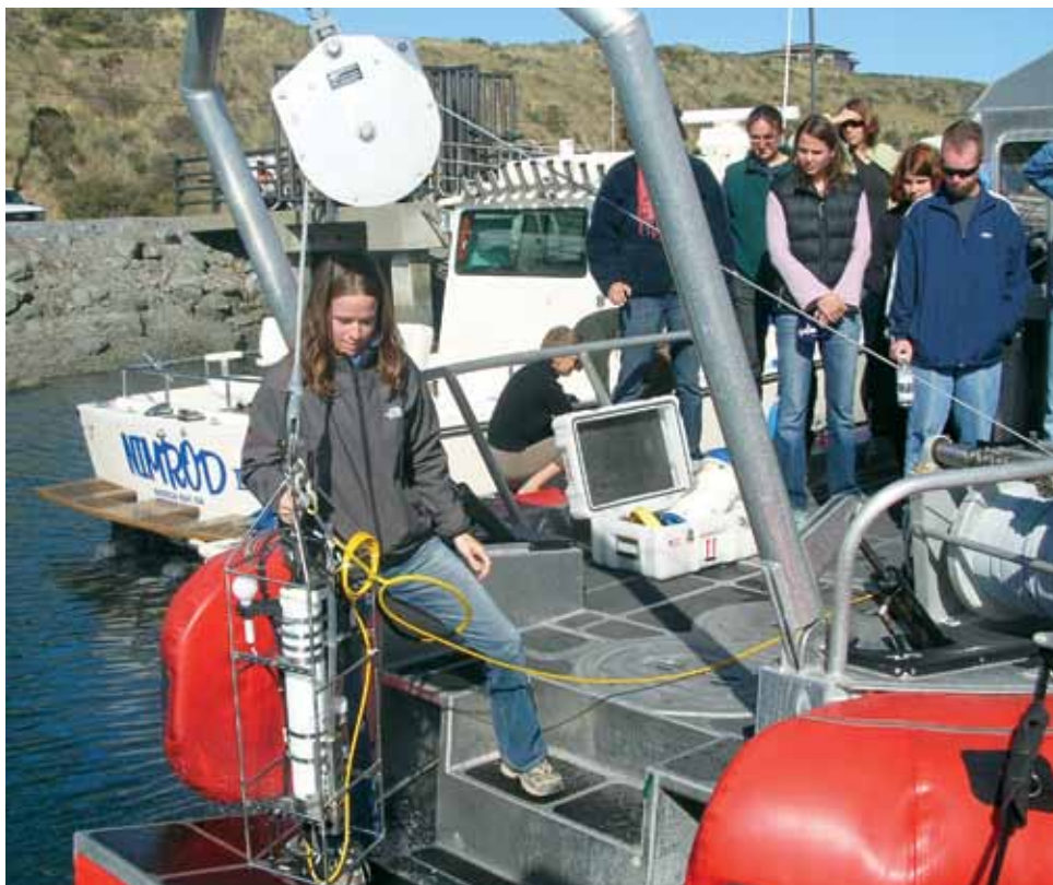
A U.C. Davis researcher deploys a conductivity-temperature-depth recorder using a winch off the back of a research vessel in Bodega Bay, Calif.
